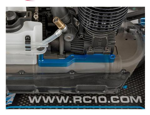
Reduce chassis flex and extend clutch bell and spur gear life in your RC8B3-series vehicle with the Factory Team Rigid Engine Mount. This extended engine mount restricts the clutch bell and spur gear area from flex, saving tooth wear and ensuring more consistent power delivery.
